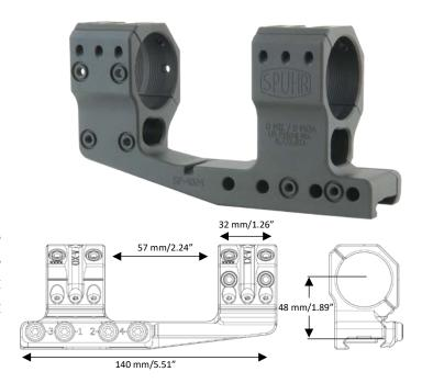
The mounts are machined from billet 7075 T651 aluminum and all aluminum parts are hardcoat anodized. The Torx 20 ring and clamping screws are zinc-nickel coated for corrosion resistance. The screws come pre-waxed from the factory to ensure proper torque values.
